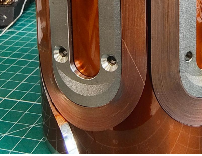
Fig. 11: Physical damage observed in the Coil 4 HTS tape, caused by accidental scalpel contact during manufacturing. Its effect on the electrical performance of the magnet is discussed in Section V-B.
