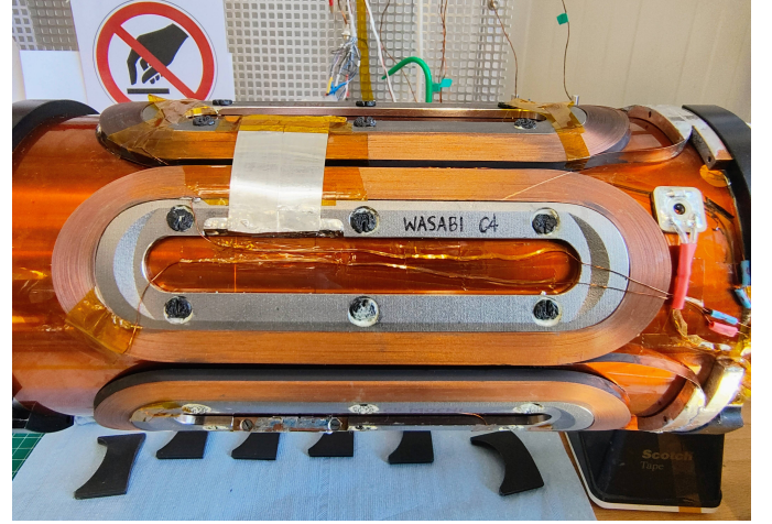
Fig. 12: View of coil showing inner and outer splice connections and voltage tap locations. Inner splices (IS) are fabricated using 12 mm HTS tape segments, while outer splices (OS) connect the coils via the outermost turns. Voltage taps enable individual coil and splice resistance monitoring during testing.
