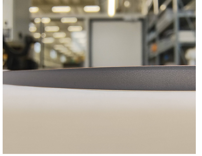
(b) Image of PVB-coated HTS tape showing the uncoated edges.
