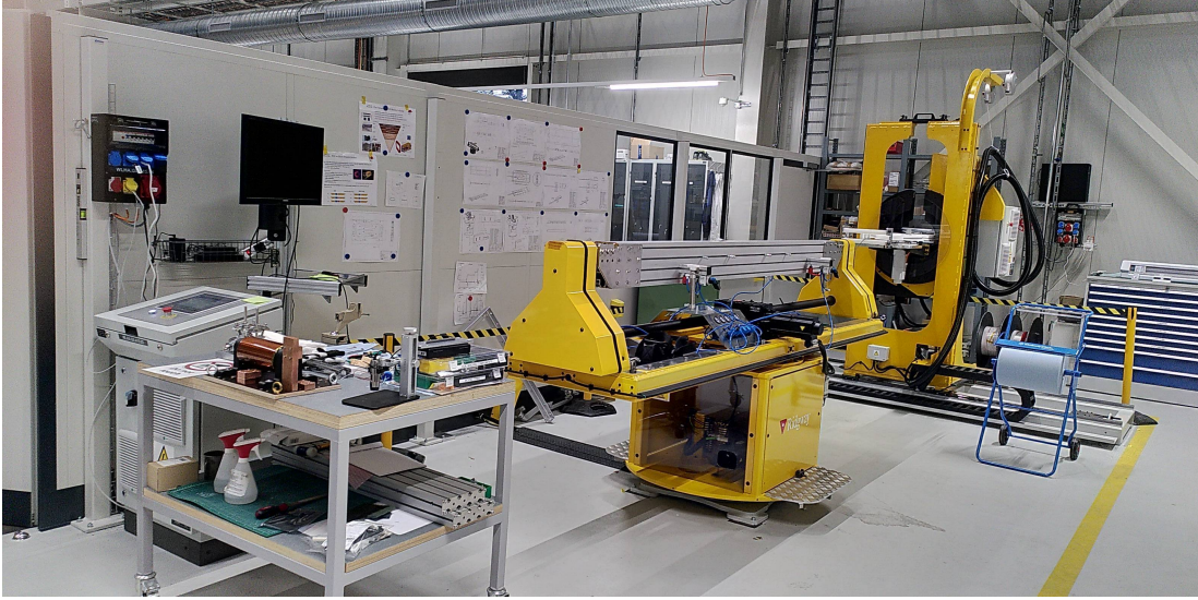
Fig. 6: 5-axis winding machine used for automated cos-theta coil fabrication, showing the coordinated control system for V-axis (vertical rotation), H-axis (horizontal rotation), X-axis (longitudinal positioning), Z-axis (vertical positioning), and R-axis (tape rotation).
