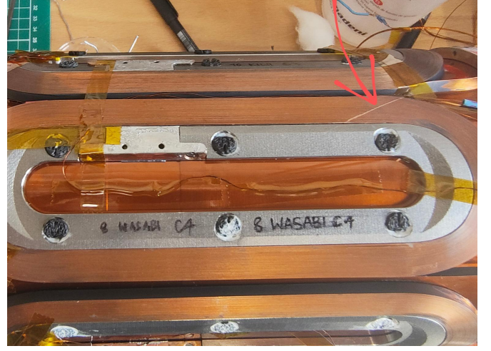
Fig. 11: Physical damage observed in the Coil 4 HTS tape, caused by accidental scalpel contact during manufacturing. Its effect on the electrical performance of the magnet is discussed in Section V-B.
