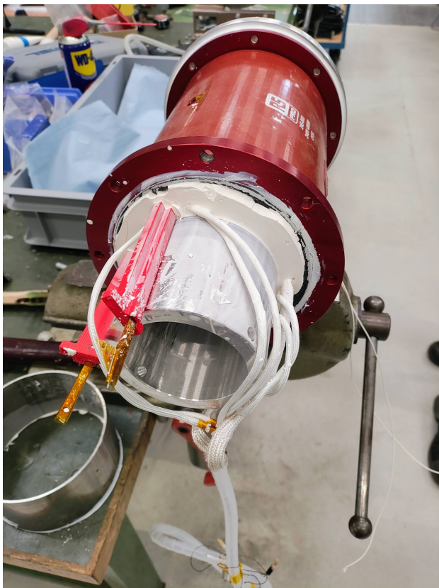
Fig. 14: Completed vacuum impregnation showing the assembly fully infiltrated with alumina-filled wax.
