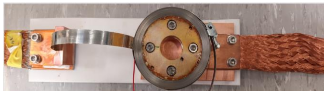
Figure 1: HTS demonstrator with tuned turn-to-turn contact resistance
