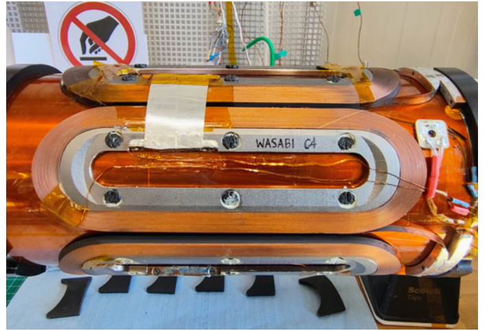
Fig. 11: View of coil showing inner and outer splice connections and voltage tap locations. Inner splices (IS) are fabricated using 12 mm HTS tape segments, while outer splices (OS) connect the coils via the outermost turns. Voltage taps enable individual coil and splice resistance monitoring during testing.
