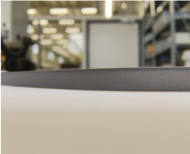
(b) Image of PVB-coated HTS tape showing the uncoated edges.
