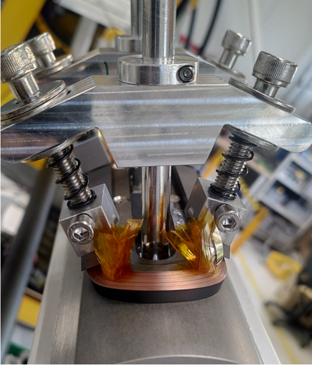
Fig. 8: Anodized aluminum clamping fixtures providing lateral support during cos-theta coil winding. The tooling is incrementally repositioned to accommodate growing coil diameter while maintaining automated winding capability throughout the 82-turn process.
