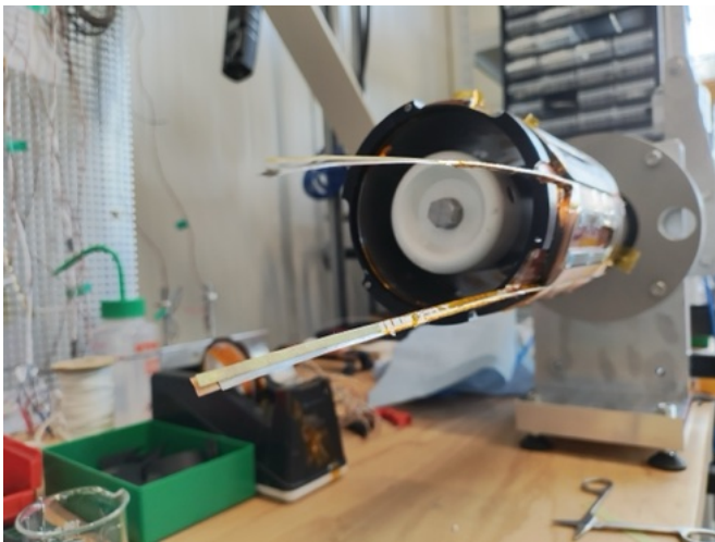
(a) Current lead assembly showing the hybrid HTS-copper conductor configuration with fiberglass mechanical reinforcement.
