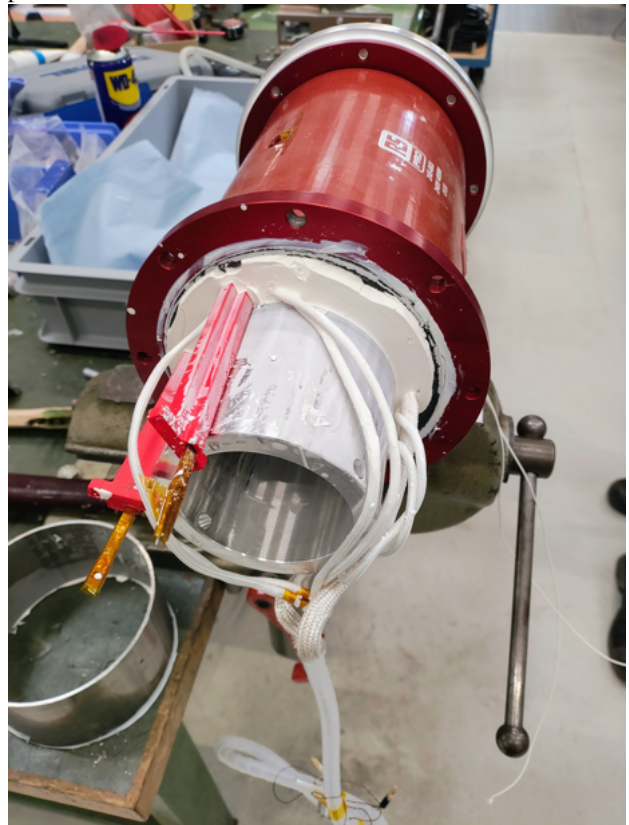
(b) Completed vacuum impregnation showing the assembly fully infiltrated with alumina-filled wax.
