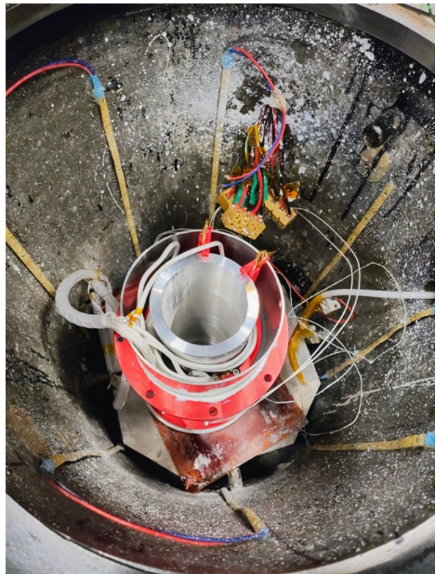
(a) Vacuum impregnation setup showing the magnet assembly positioned within the vacuum chamber.
