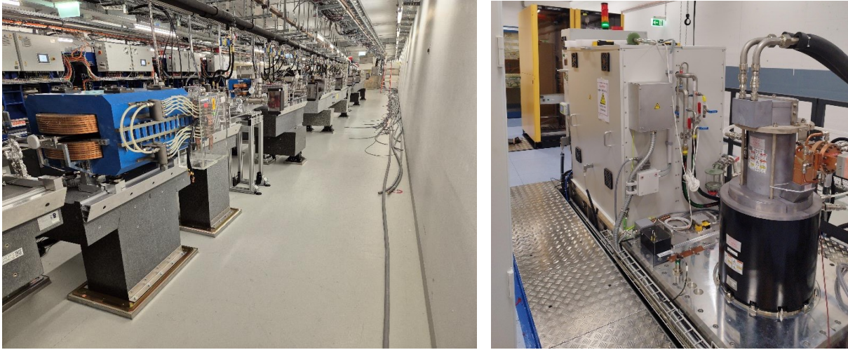
Figure 17: Left: P^3 beamline installed in SwissFEL. Right: RF modulator in the technical gallery.
