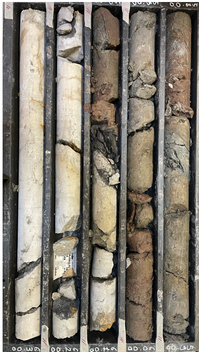
Figure 5.4. Mandallaz 2 core displaying the 97-millions years gap unconformity between the lower Cretaceous limestones and the Oligocene Molasse). The carbonates consist of the “Urgonian” micritic white limestones while the Molasse consists of clastic deposits associated with continental depositional environment.
