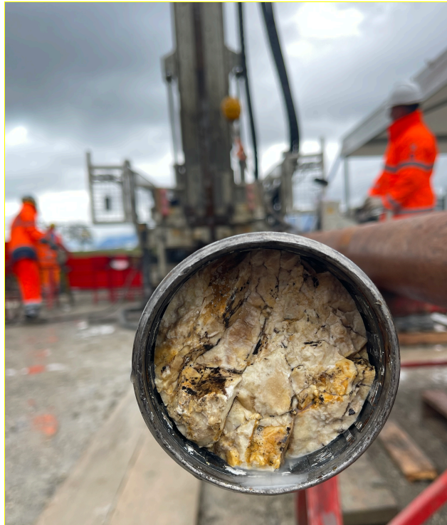
Fig. 5.1A – Photograph of the core barrel immediately after recovery at the surface of borehole MAND_02, showing a portion of the Lower Cretaceous limestone ("Urgonian" Facies).
