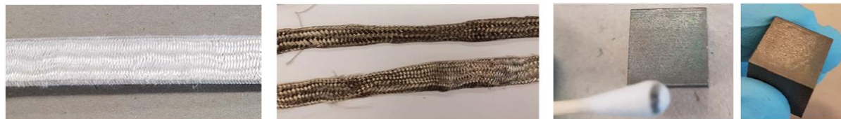
Figure 14 From left – (2): Glass-fiber braid before and (2) after reaction cycle, the pyrolysis of the glass-fiber sizing leads to conductive residues on the braid and contaminates nearby surfaces (3 and 4).
