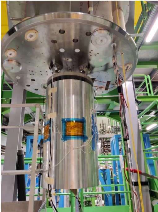
Figure 3 Left: CD1 magnet on the header of the test station at CERN. Right: Testing team in the control room of SM18 at CERN: Michael Daly (PSI), Daniel Molnar, Jean-Luc Guyon, and Franco Mangiarotti (CERN).
