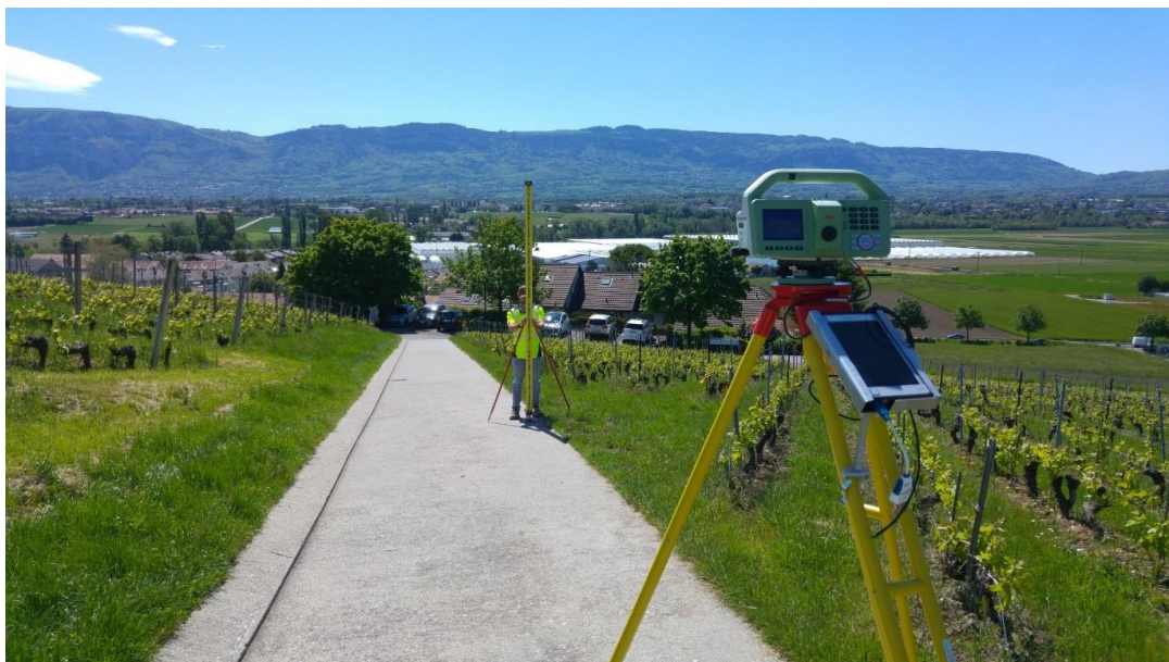
Figure 7: View of the sloping Bernex's vineyards, the PDA acquisition device is connected to a Trimble DiNi03.
